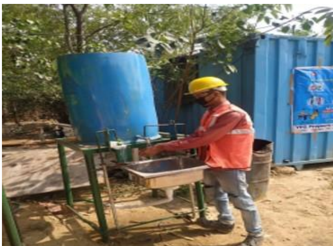
The foot driven hand washing facility installed at Delhi Metro's construction site
